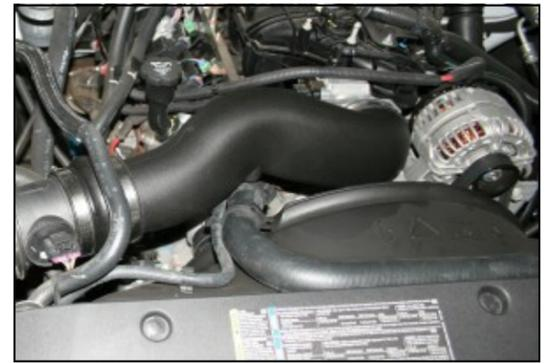
**12.** Install the Airaid Intake Tube into the hump hose first, and then onto the throttle body. Adjust it for fit, and then tighten the hose clamps.
