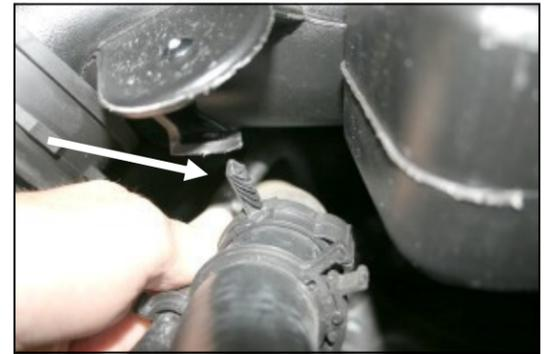
3. Separate the factory intake tube from the plastic clamp that secures the radiator hose to the tube. A firm downward push will usually do it.
