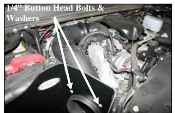
6. Slide the Airaid Intake Tube (#2) into the CAB first, and then into the hump hose. *If needed, the factory turbo intake tube can be adjusted for proper alignment.* Next install four 1/4" button head bolts (#6), and four flat washers (#7) thru the CAB to secure the Airaid Intake Tube. Now tighten the three bolts at the bottom of the CAB and the two hose clamps on the hump hose.
