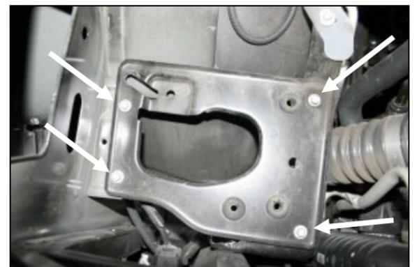
3. Using a 10mm socket, remove 4 bolts, and remove the factory air filter mounting plate.
