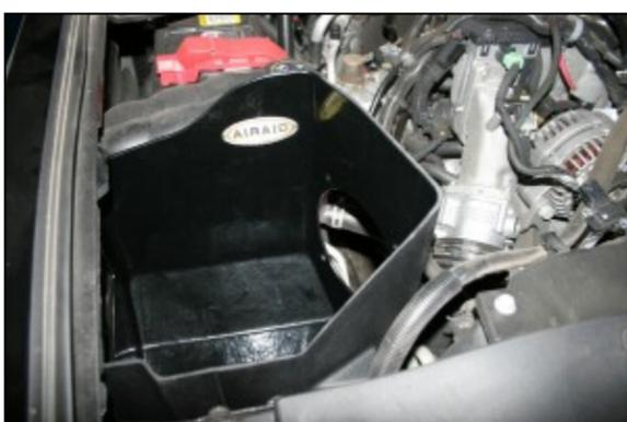
4. Install the Airaid Cool Air Box (CAB) (#3) into the vehicle as shown, replacing the factory air filter. Install three M6-1 x 25mm bolts (#9), and three flat washers (#7) thru the bottom of the CAB and into the factory captured nuts. Leave the bolts loose for now. Apply the Airaid Bubble Decal inside the Airbox as shown.
