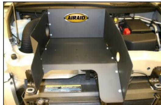
**6.** Assemble the three **Cool Air Dam** panels (#2, #3, & #4), using 13 screws (#11), washers (#12), and nuts (#13). Apply the Airaid Foil Decal onto
