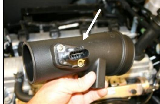
**9.** Install the **Mass Air Flow** sensor removed in step #4, into the Airaid Intake Tube (#5) using the two 8/32"x 3/8" button head screws (#10). **DO NOT USE THE FACTORY SCREWS!**
