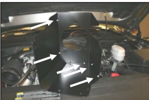
7. Assemble the two Cool Air Dam panels (#2) and (#3) as shown, using the five 6-32 screws (#10), washers (#11), and nuts (#12)
