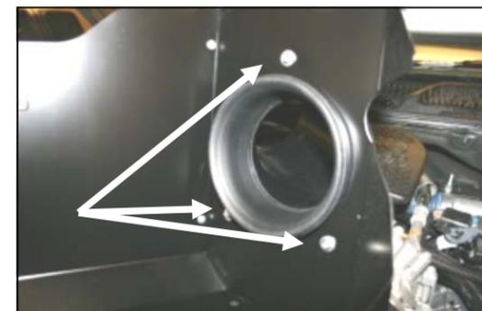
8. Install the Airaid intake tube (#4) into the Cool Air Dam using the three 1/4"-20x1/2" button head bolts (#6), and washers (#7) as shown.
