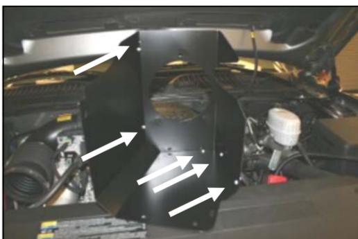
7. Assemble the two Cool Air Dam (CAD) panels (#2) and (#3) as shown, using the five 6-32 screws (#10), washers (#11), and nuts (#12).
