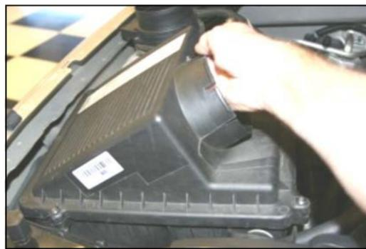
5. Grab the factory airbox and rock it back and forth, and remove it from the vehicle. It is only held in by grommets, no bolts.
