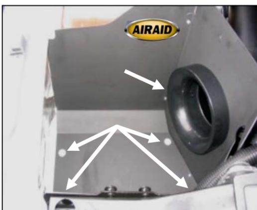
**7.** Install the air filter adapter (#4) using three 1/4-20x 1/2" button head bolts (#12), and 1/4" flat washers (#13). Position the Airaid Cool Air Dam in place of the factory airbox & secure it with four M6-1x25 hex bolts (#14) and 1/4" flat washers (#13).
