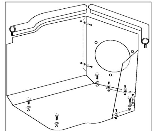
**6.** Assemble the Airaid Cool Air Dam panels (#2, #3) using five 6-32x 5/16" screws (#9), #6 flat washers (#10), and 6-32 keps nuts (#11).
