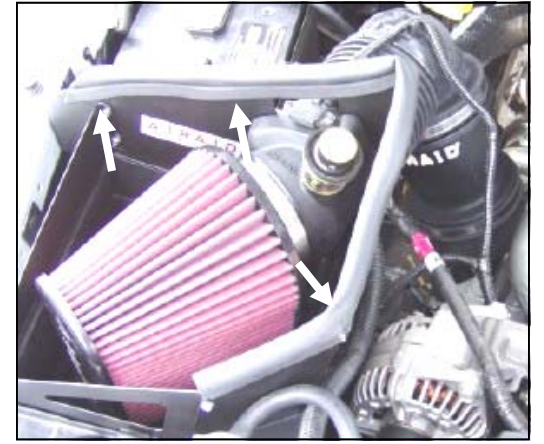
15. Install the Airaid Premium Filter (#1) onto the air filter adapter. Install the weather strip (#6) onto the top of the CAD. (Hint: start at one end, and work to the other).
