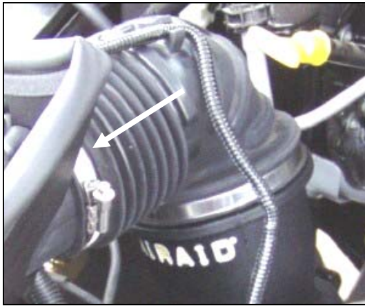
13. Slip the intake tube onto the air filter adapter, and tighten the clamp.
